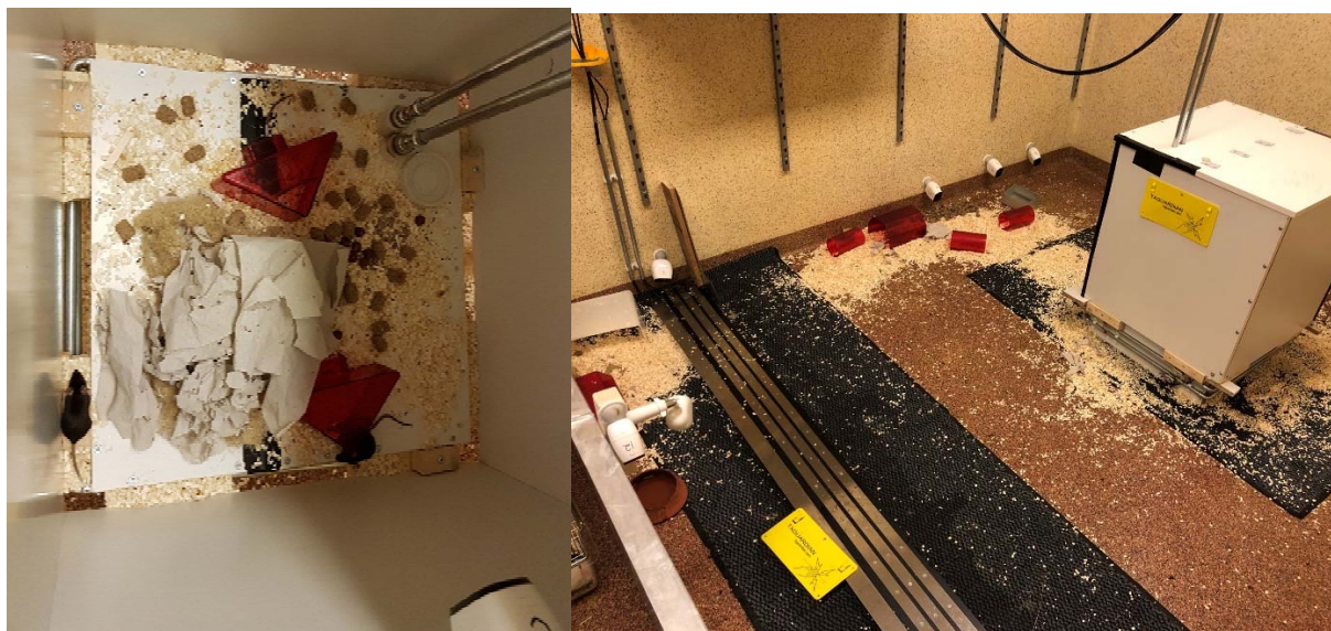
Figure 2. The left photo shows mice inside the test house with food, kernels, water, red plastic shelters and nesting material. On each side there is a slot for entrance/exit. The metal pipes which can be electrified (only visible to the left) are used by the animals to climb on to get inside. The photo to the right shows the test area with the carpet underneath the test house and floor list (installed to improve conduction) and placement of enrichments (here in rat size) and feed/water. Photo: Cecilie Mejdell.
