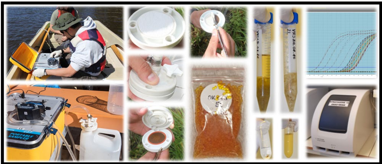
Figure 4. Water samples of ~5 L each were filtered on-site through glass fibre filters using a portable peristaltic pump (Masterflex E/S portable sampler). Each filter was carefully transferred to a 15ml tube with buffer and stored there, until further processing in the laboratory. DNA was isolated with a large volume extraction procedure and presence/absence of eDNA from all target organisms was analysed using qPCR. Figure modified from Vrålstad et al (7).
