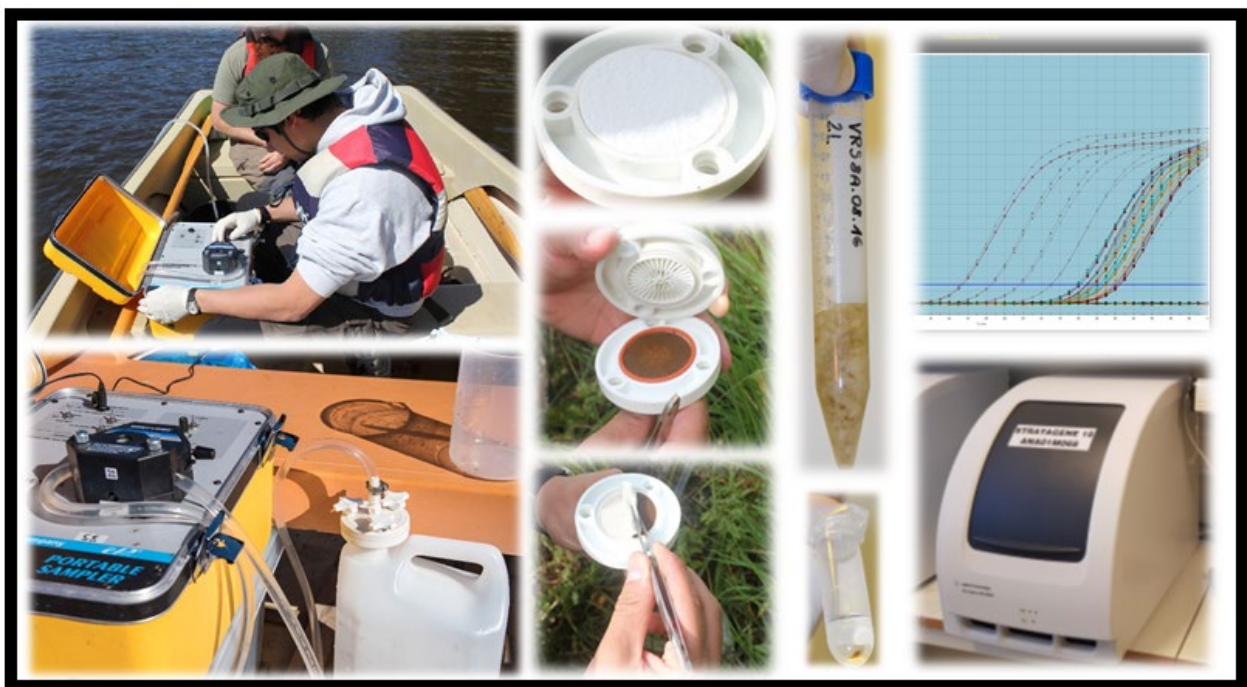
Figure 4. Water samples of ~5 L each were filtered on-site through glass fibre filters using a portable peristaltic pump. Each filter was carefully transferred to a 15ml tube with buffer and stored there, until further processing in the laboratory. DNA was isolated with a large volume extraction procedure and presence/absence of eDNA from all target organisms was analysed using qPCR. Figure modified from Vrålstad et al. 2016 [7].
